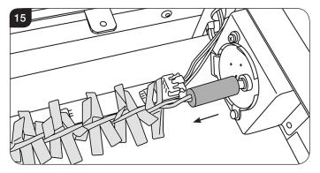
7.5 Withdraw the spindle from the left hand bracket, see Diagram 16. The spindle may need to be tilted to be removed from the location bracket.
