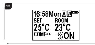
If the heater is on in the current period, pressing the button will turn the heater off.
