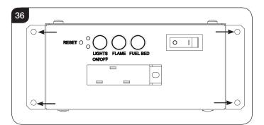
15.3 Support the Power Unit and remove the 4 screws.
