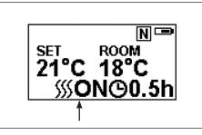
Note: It is normal for the fan heater to stop running for periods of time. This happens if the room temperature is higher than the temperature set on the control.
