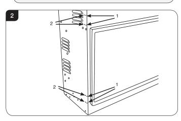
3.2 Attach the 4 fixing brackets to the sides of the appliance, see Diagram 3.
