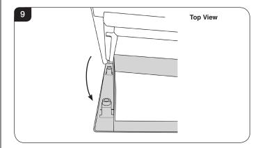
4.3 There is a clamp at the top of each corner of the glass viewing panel that secure the glass in place, see Diagram 10.Take care to support the glass when removing clamps.
