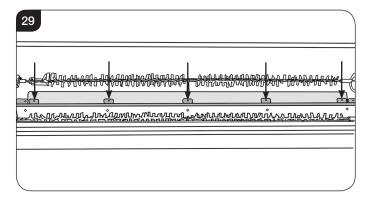
NOTE: When refitting the shield ensure that the lip curves down and towards the back. It will be necessary to lift the shield slightly to align the screws. Refit the screws from inside out. 12.3 The LED boards are located below the Effects Spindle, see Diagram 30.
